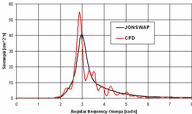
Figure 3. Comparison between theoretical JONSWAP spectrum and actual spectrum of the wave obtained in CFD
