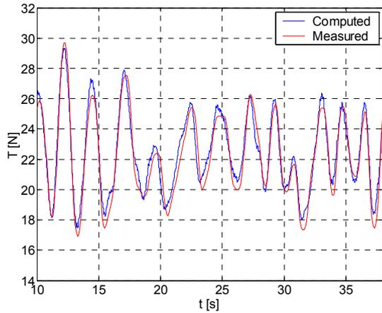
Figure 10. Computed vs. measured tension of mooring tether
