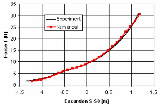
Figure 5. Comparison between computed and measured static characteristics of the mooring tether.
