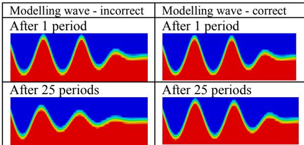
Figure 2. Modelling the regular waves
