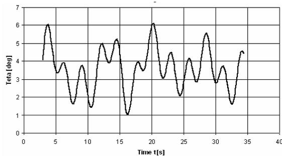
Figure 11. Pitch angle in regular wave, computed with CFD
