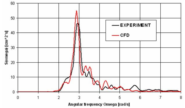
Figure 12. Wave energy spectra – CFD vs. experiment
