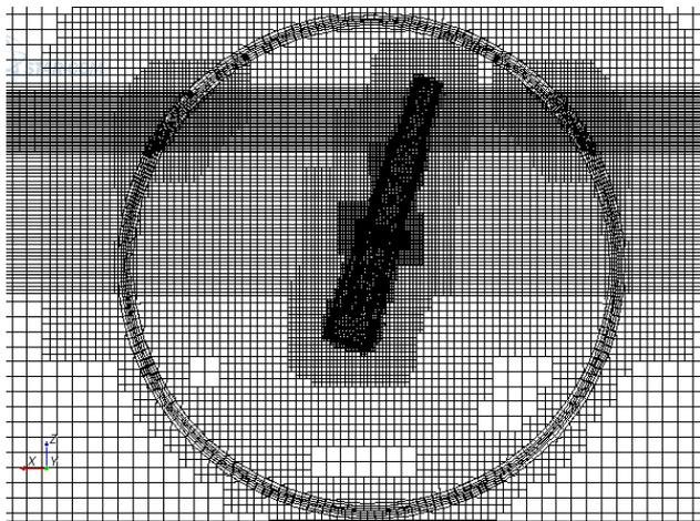
Figure 6. Computational mesh details
